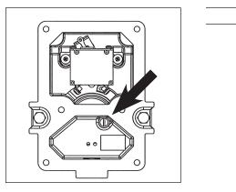
Using wire nuts, connect the black wire to the black wire and the white (or red) wire to the white (or red) wire in the pump's electrical cavity. Position the wires inside the electrical cavity and tighten the strain relief grip securely. Make sure surfaces are clean. Install the coverplate and tighten securely.
