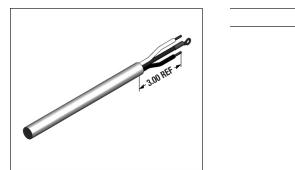
Insert the power cord through the 3/4 inch NPT connection on the bottom of the pump. Attach ground wire (green) using green ground screw located inside the electrical cavity. (Figure 3)
