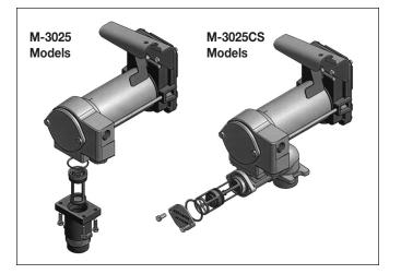
Turn the pump off and disconnect from power. Depending on the model, remove and clean the strainer with a soft-bristled brush and solvent. If the strainer is very dirty, compressed air may be used. If damaged, replace the strainer.
